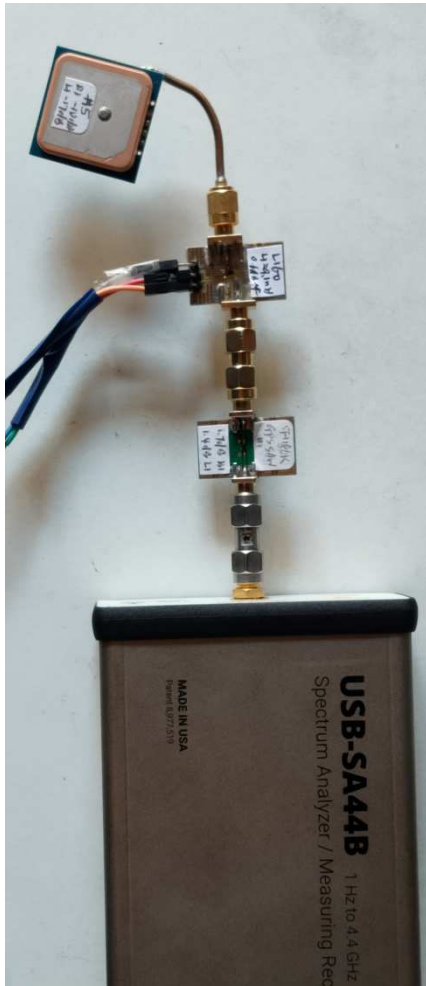
SA: Signal Hound USB-SA44B, Range 1555-1615MHz RBM=VBW=10KHz, MaxHold
