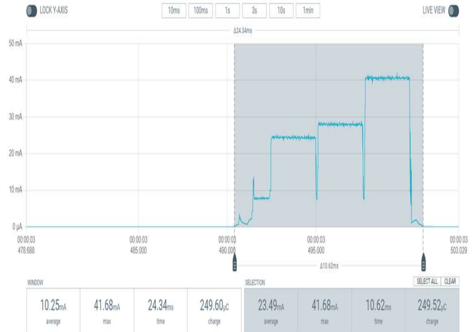
DUT BHW#16, Coded PHY 125K (S=8) 69.3nAh or 249.5uC per Beacon Event
