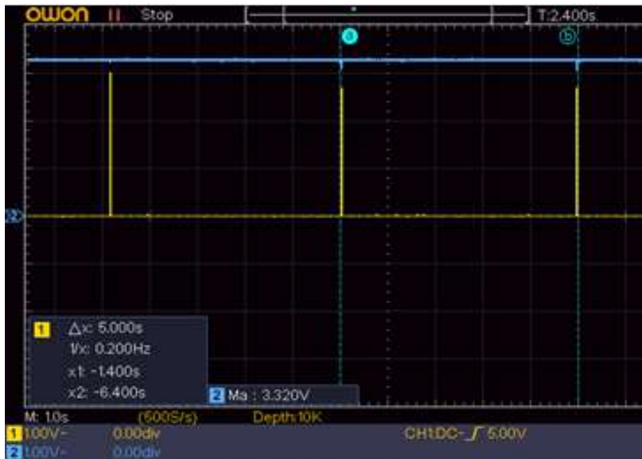
Example SW0 Waveform Advertising Interval 5 sec
