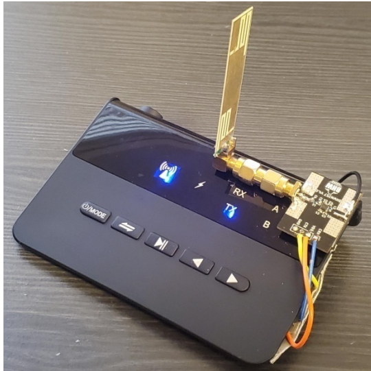
Receiver: Qualcomm CSR8675 BLE SoC + BHWM257 FEM + BHWR250 Antenna
