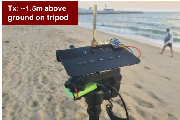
Transmitter: Qualcomm CSR8675 BLE SoC + BHWM257 FEM + BHWR250 Antenna
