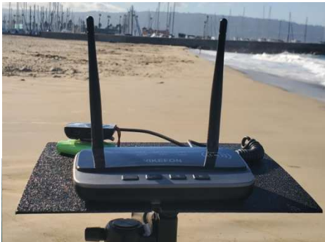
Original Unit without Modification: Antenna in Vertical Orientation
