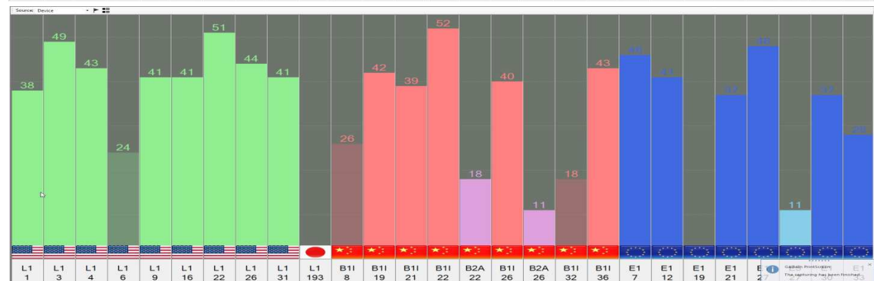
Antenna Rotated by 90 Degree Max. C/N0=52dB
