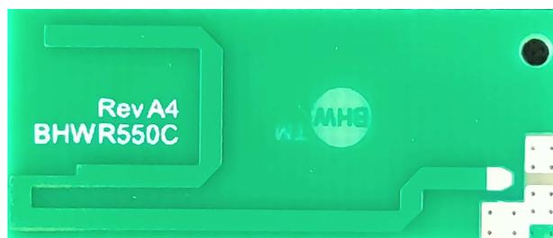
12x30x0.6mm PCB for IPX/UFL Cable Assembly
