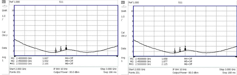
DC bias: Vdd=CRX=3.3V, CTX=0V. VSWR may vary slightly for different main PCB thickness/material/size/shape and plastic housing designs, but should be significantly less sensitive than conventional small antennas.
