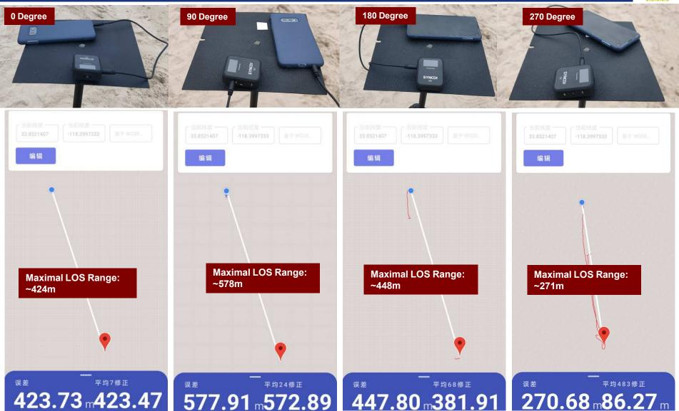
RX unit was placed behind the neck to emulate LOS test condition when walking away from TX. Maximal range was recorded when music streaming started to break down. Average value for Max Range from 4 different Tx antenna angles was 430m.
