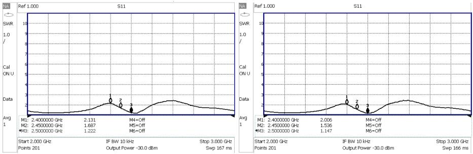
DC bias: Vdd=CTX=3.3V, CRX=0V. VSWR may vary slightly for different main PCB thickness/material/size/shape and plastic housing designs, but should be significantly less sensitive than conventional small antennas.
