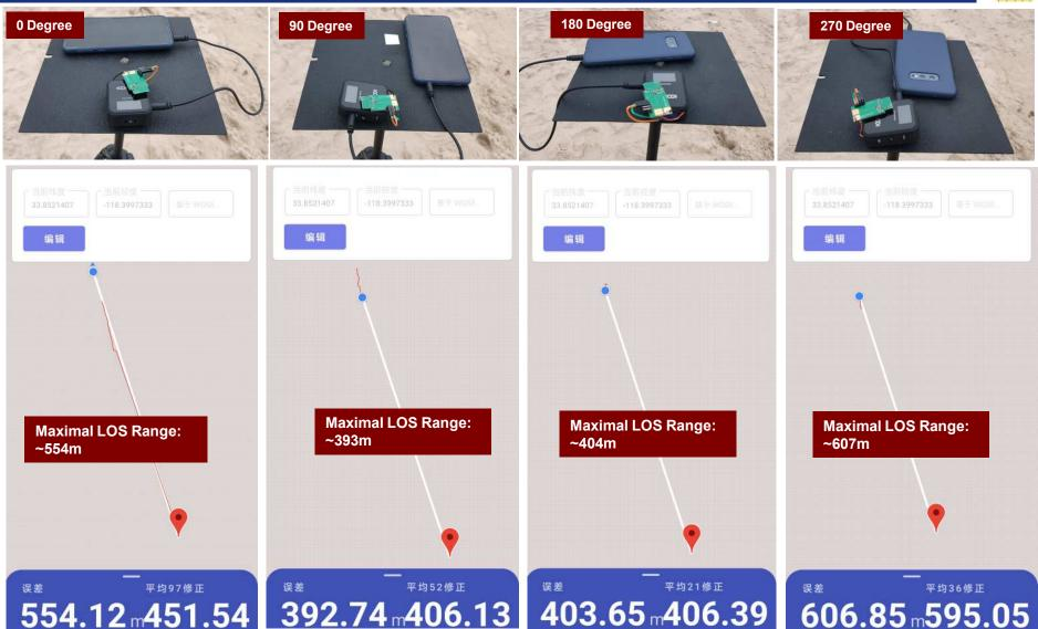
RX unit was placed behind the neck to emulate LOS test condition when walking away from TX. Maximal range was recorded when music streaming started to break down. Average value for Max Range from 4 different Tx antenna angles was 489m.
