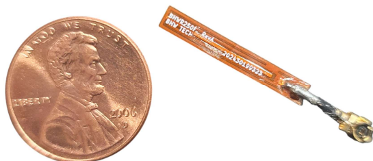
3x20x0.2mm Flex PCBA with IPX/UFL Cable Assembly
